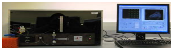
Ciencia's Dual mode SPR Fluorescence Analyzer
